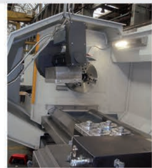
"Power Grip" system with replaceable units for quick change tools system
