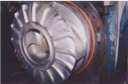
millMAX™ after 1500 hours of wear
