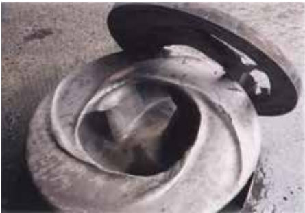
Competitor's suction liner and impeller - 550 hours
